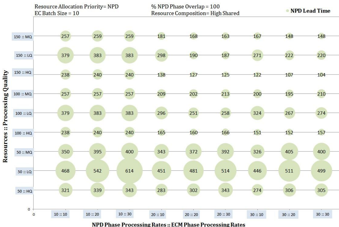
Figure 42: Influence of resources and processing quality, and NPD and ECM processing rates on NPD
